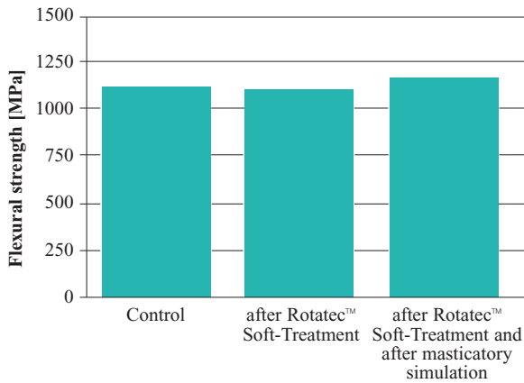
Fig. 5.4: Weibull strengths of Lava™ Frame zirconia after treatment with Rocatec™ Soft and after additional masticatory simulation (50N, 1,2 millions cycles + Thermocycling 5°/55°, 3800 cycles).
