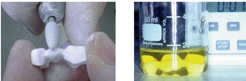
Fig. 2.5: Manual finishing before sintering(a),, Coloring of Lava™ Frame zirconia framework before sintering (b)
