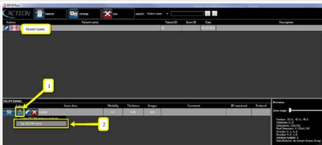
Step 2: When the CBCT loads, click the folder icon found under “DICOM Series”, then click “Zip DICOM series”.
