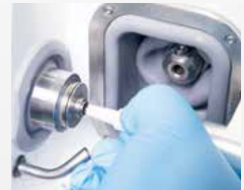
Step #8 – Clean tapered spindle shaft
