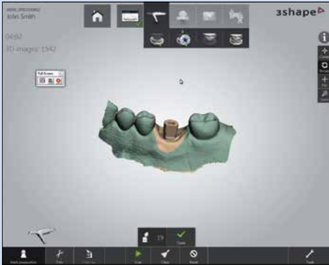
When scan is complete, press #19 icon then press the scan abutment
